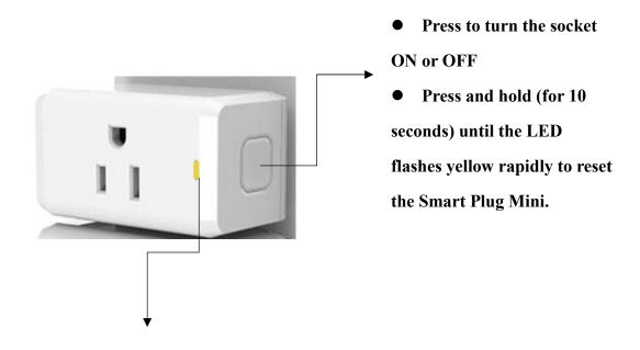
Flashing blue rapidly: After the configuration is successful, the specified WiFi router is being connected
